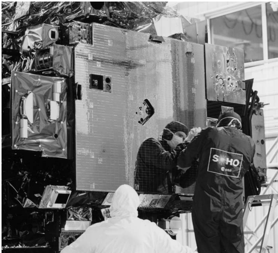
FIGURE 18. Photo of the Sun-facing part of the SOHO spacecraft where VIRGO is integrated. The largest opening is the LOI instrument.
