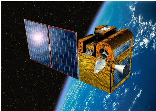
Fig. 1: Artist view of PICARD microsatellite, 60x60x80 cm<sup>3</sup> in size. Shown are the 3 instruments of the payload: SODISM, telescope and guiding, right, SOVAP, differential radiometer, center, and PREMOS (flux monitors) left, near the solar panels. In the back, one can see the electronics box supporting two S-band antennae and a solar pointer (acquisition maneuvers).
