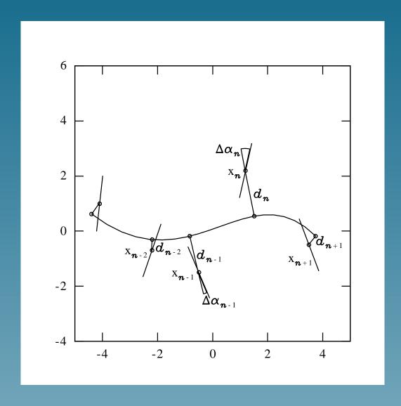
The smoothing spline is constrained by the minimization of:
