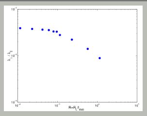
The perpendicular mean free path: simulations and nonlinear theory of Shalchi et al. 2004. The QLT-result is  $\lambda_{\perp}/\lambda_{\parallel} = \infty$ .
