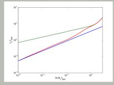
The parallel mean free path in the interstellar medium: quasilinear result in comparison with a  $R^{0.6}$ -fit and the nonlinear result from Shalchi & Schlickeiser (2005).
