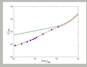
The parallel mean free path: simulations, quasilinear theory, and nonlinear theory of Shalchi et al. 2004.
