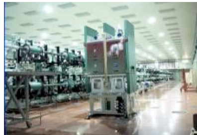
FIREX 1 Osaka Japon 10 kJ 2 \omega_0 + 10 kJ - 1 PW
